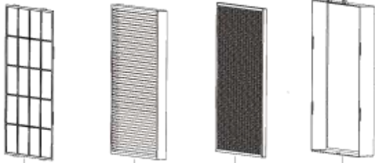
Coarse Filter HEPA Filter Carbon Filter Filter Assembly Compartment
